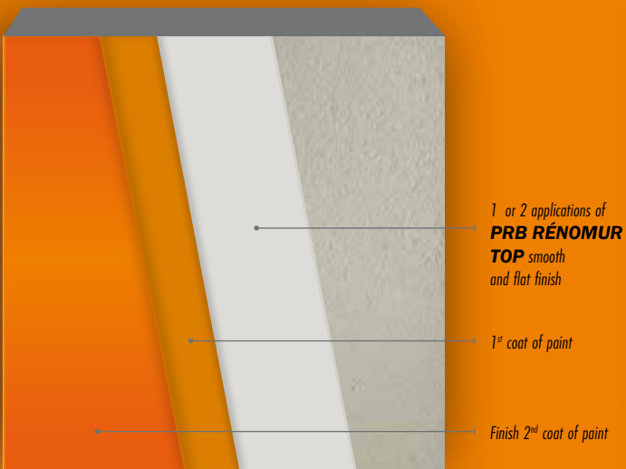
Healthy unpainted substrate (no cracks and flaking)
