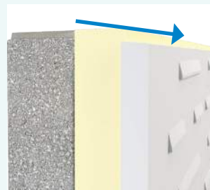
Edging sloped towards outer leaf to ensure wall ties sloped down
